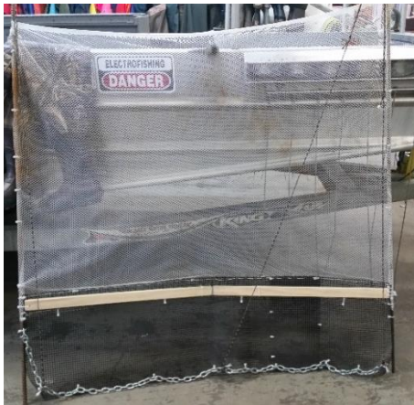
Preliminary design for the structures in 2016. The wood support was removed and the chains were replaced with 2" diameter sandbags.
