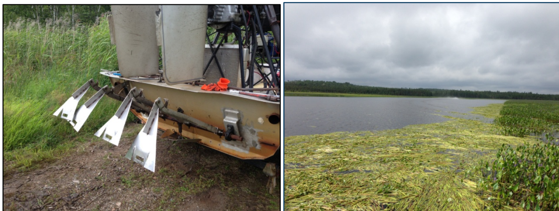
Figure 9. An example of equipment used by FdLNR to reduce existing vegetation prior to wild rice seeding. (Photo courtesy of FdLNR).
